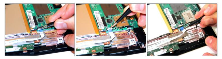
• Lift up the power button cable retention clip on the motherboard and pull the cable out.
