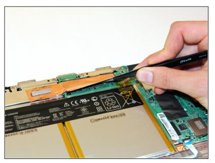
• Remove the copper tape carefully.
