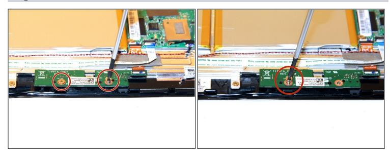
• Remove the two screws on the camera board using a Phillips #1 Screwdriver.
