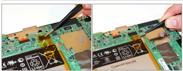
Gently pull back the yellow transparent plastic covering on top of the battery connection port.
