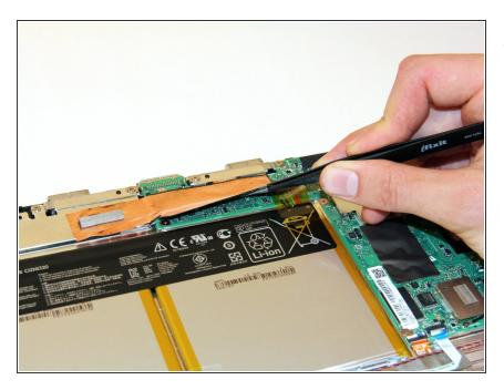
Remove the copper tape carefully.
