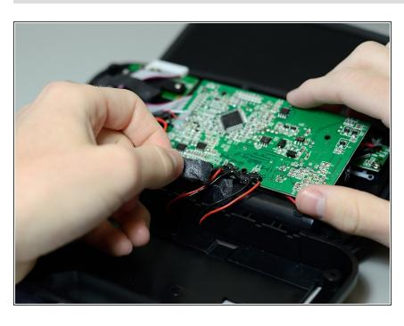
Peel away the black tape covering the red wires that connect to the PCB.
