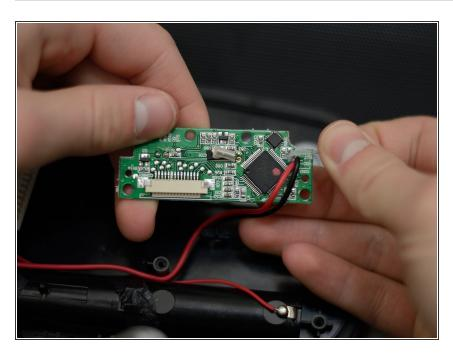
Peel away the glue connecting the red and black wire with the PCB board.
