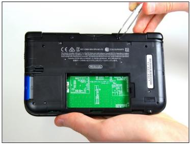
• Using <u>tweezers</u> pull out the rubber bumpers that are located at the top of the device on either side of the game cartridge compartment.
