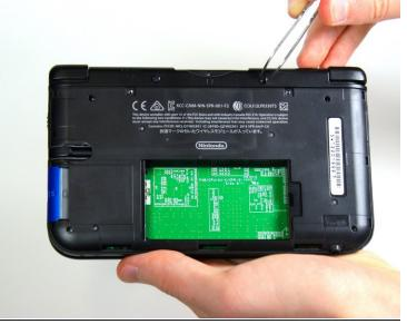
Using tweezers pull out the rubber bumpers that are located at the top of the device on either side of the game cartridge compartment.
