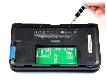
Remove the six 6.2 mm screws using a Phillips #000 screwdriver.
