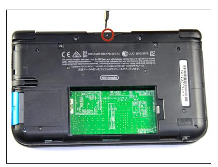
Remove the 2.3 mm screw located above the game cartridge slot with a Phillips #000 screwdriver.
