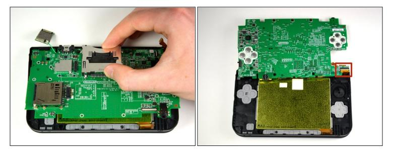
The motherboard will still be attached at the top right hand corner so do not completely detach it at this point.
