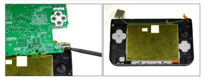
• Using the flat head side of the spudger carefully lift up the flap that attaches the wider ribbon on the upper right side to the motherboard.
