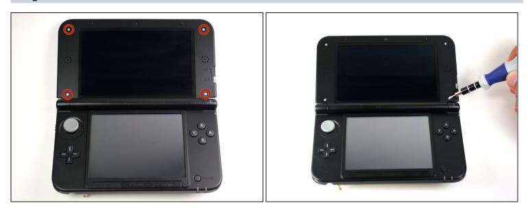
• Remove the four 4.3 mm screws located underneath the four rubber pieces with a Phillips #00 screwdriver head.
