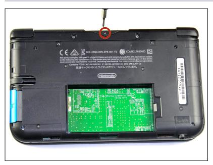
Remove the 2.3 mm screw located above the game cartridge slot with a Phillips #00 screwdriver.
