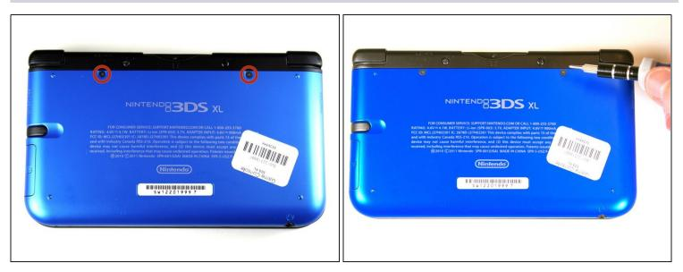
Loosen the two #0 Phillips 4.2 mm-length screws located at the top of the back cover.
