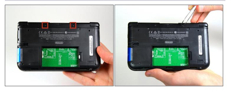
• Using <u>tweezers</u> pull out the rubber bumpers that are located at the top of the device on either side of the game cartridge compartment.
