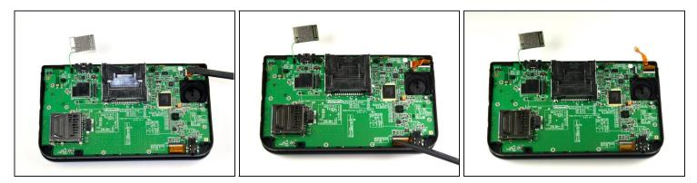
• Using the flat head side of the spudger carefully lift up the flaps that attach the wider ribbons to the motherboard.
