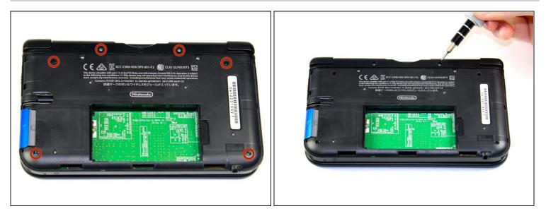
• Remove the six 6.2 mm screws using a Phillips #00 screwdriver
