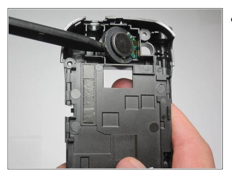
Using a spudger, remove the speaker
