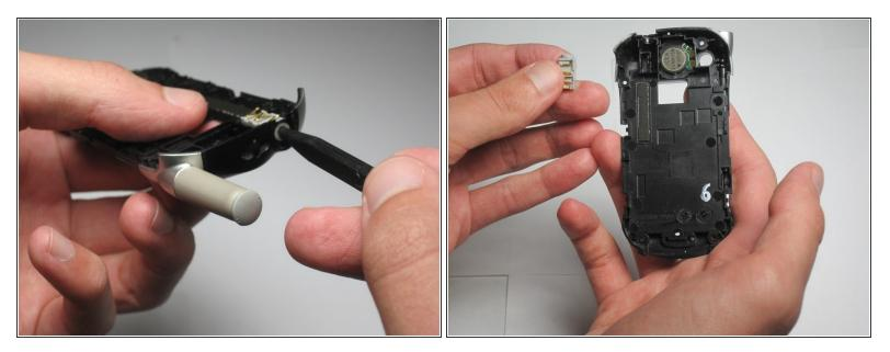
On the back casing, using a spudger, push into the headphone jack at an upward angle to pop it out
