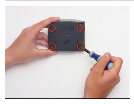
Use a T-9 Torx screwdriver to unscrew the four screws on the back cover.
