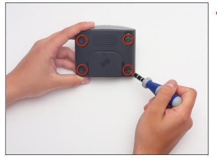
• Use a T-9 Torx screwdriver to unscrew the four screws on the back cover.
