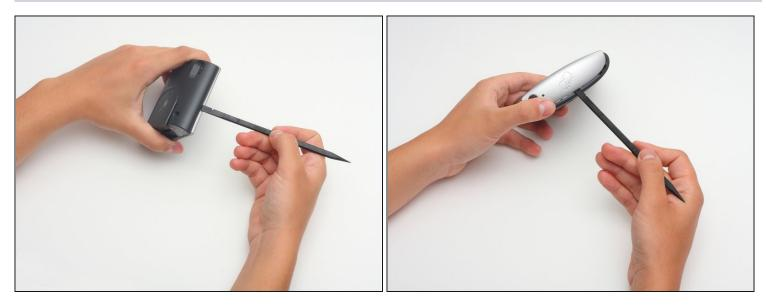
• Using a spudger, gently pry apart the back case from the front case. It is easier to start on a side and work your way around the device.
