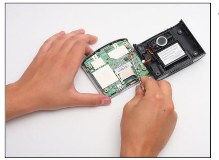
Once the two covers are separated, use the <u>tweezers</u>, or even your fingers, to gently disconnect the two sets of wires that are connected to the motherboard from the back cover. You may have to wiggle the wires a little bit to get them to disconnect.
