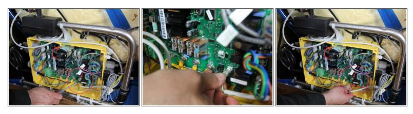
Disconnect the plug from the pressure switch
