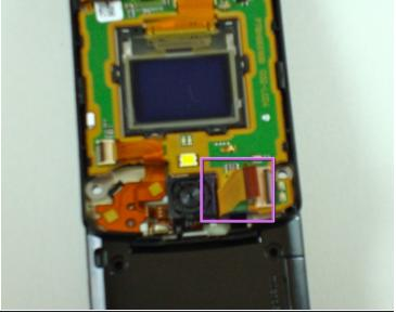
Firmly grab the flexible circuit with tweezers to detach (or use your fingers if you can manage a firm grip).
