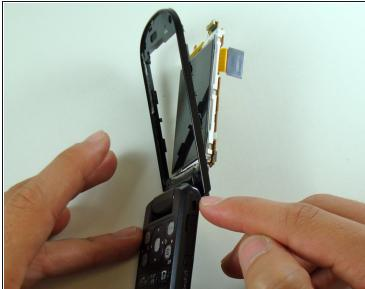
The LCD screen and circuit board should now be partly detached from the frame.
