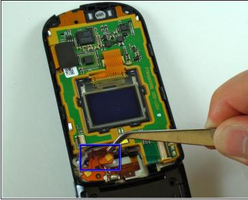
Remove the flexible circuit shown using tweezers (or use your fingers if you can manage a firm grip).
