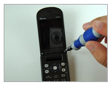
Remove the screws using a Y0 screwdriver.
