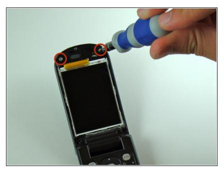
• Use the Y0 screwdriver to remove the screws.
