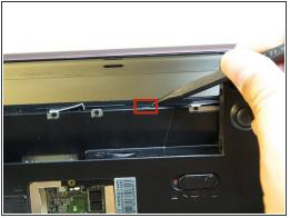
Release the 3 black clips by pushing them in with the pointed end of the spludger.
