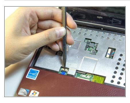
Remove the ribbon cable that is connected to the circuit board with the pointed end of the spudger.
