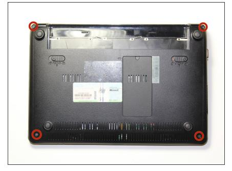
Remove the four 6 mm screws with the Phillips #1 screwdriver.
