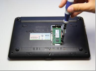
Locate and remove the silver 6.65 mm Phillips #1 screw in the bottom right corner of the opening.
