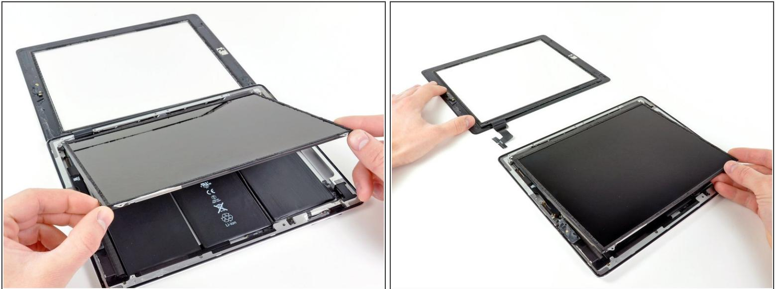
**i** In order to remove the front panel assembly, the ribbon cable needs to slide out between the case and the LCD. You'll need to move the LCD to make some room.
