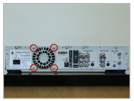
The fan is held in by four T15 screws on the rear of the device.
