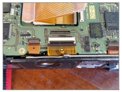
The two middle cables need to be removed next. Use the same process as before, or if no tightening bar is present, gently pull the cable straight out.
