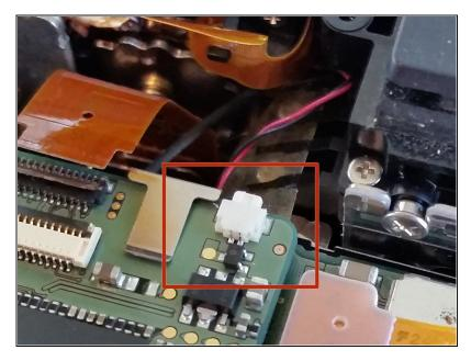
The red and black power cable can be removed next. It it different than the rest, and can be removed by either using a plastic opening tool or a very small pair of pliers to remove it.
