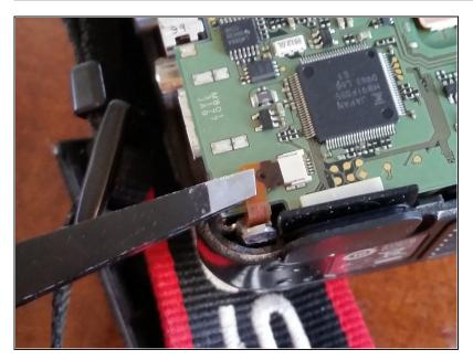
Next to remove is the bottom left corner flex cable. It has no tightening bar, so pull it out with tweezers or with your fingers.
