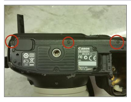
Three screws on the bottom need to be removed next. They can be removed in any order
