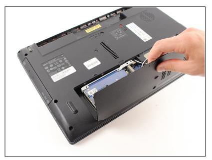
After the panel has been loosened by the plastic opening tool, take your finger, place it in the gap, and remove the panel from the laptop.
