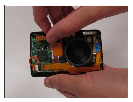
Using a Phillips #00 screwdriver remove the single screw on the far left-hand side towards the bottom of the camera.
