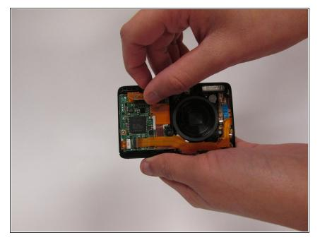
Remove the front panel of the camera case to expose the top left ribbon cable. Pull the ribbon cable gently to disconnect it from the camera.
