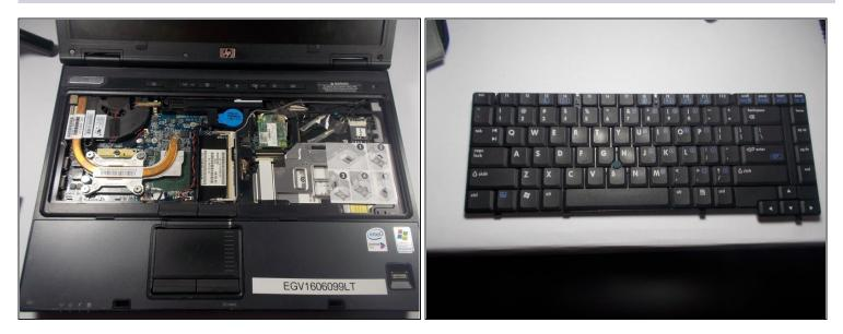
• At this point the keyboard should be completely detached and ready to be removed. Be sure to take your time installing the ribbon cables as these can be troublesome if not installed properly
