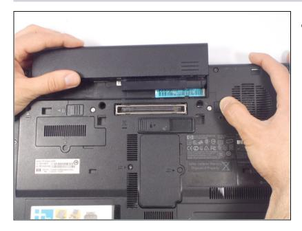
• Once both the battery locks are unlocked, slide the battery out to remove.
