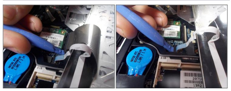
• Now with <u>tweezers</u> or a gentle prying apparatus gently pull the lock on the retaining clip up to release each ribbon cable. It is important to only pull up on the lock and not the entire clip.
