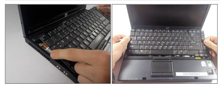
• At this point the back of the keyboard should come up a bit. You may need to use a thin tool to pull it up, but in my case I only needed my hands. Once you have the back of the keyboard propped up as shown pull the keyboard gently towards the screen to remove. Be careful not to pull completely out because there are still connectors attached to it.
