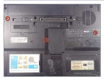
• Locate and remove the 3 screws holding the keyboard in place from underneath the laptop.
