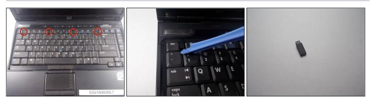
• Locate and remove the four retaining clips from the edge of the keyboard. To remove pry up gently on the outside edge of the plastic clip. Once the clip pops up pull it straight out.
