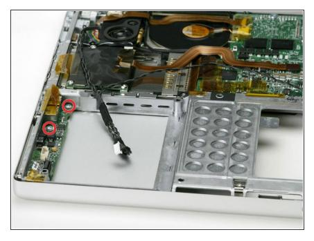
Remove the two T8 Torx screws from the sound board.
