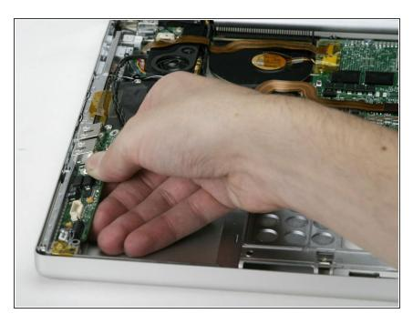
Grasp the sound card near the ports and pull it out, rotating it clockwise to work around obstacles.
