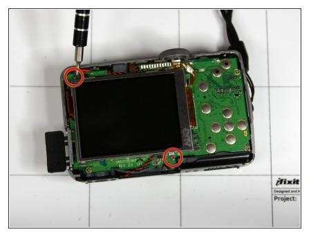
Remove two screws holding screen to circuit board marked by red circles
