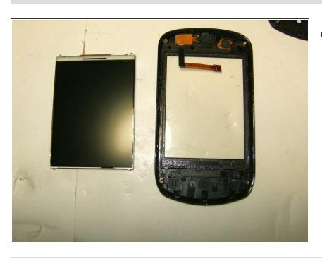
Here is the LCD removed. LCD and Digitizer are separate piece which makes the a economical feasible repair.
