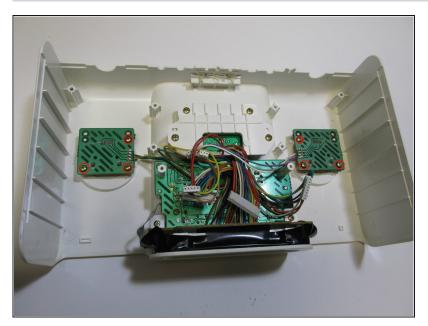
Remove the three screw from the dial with a #2 Phillips screwdriver.
