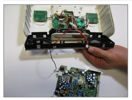
Remove the front piece by pulling up until it hits the plastic pieces sticking out from the display screen. Then pull it out horizontally from the device.
