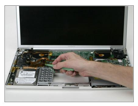
• Disconnect the orange hard drive ribbon from the logic board.
