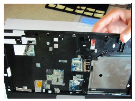
• Lift off the top cover and remove it. Lift off from the back.
