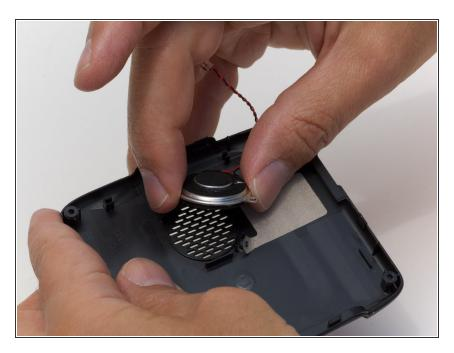
Once the speaker has been unscrewed, remove the speaker from the back casing with your fingers.
