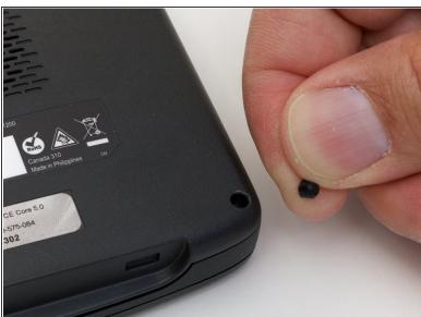
Remove the four rubber caps from the back by using the Phillips #00 screwdriver.
