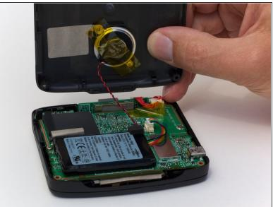
Remove the back cover from the device by separating the back cover along its seam.
