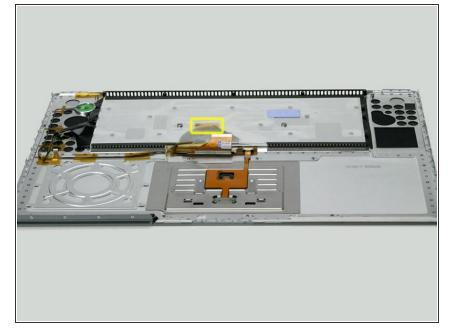
• Remove the orange tape that covers the keyboard connector and ribbon.
