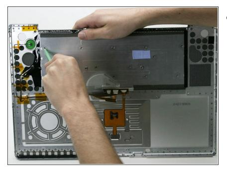
Place the upper casing on edge and use a spudger to push the keyboard away from the casing, poking the spudger through the holes where the screws were.
