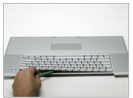
Lay the casing flat so that the keyboard faces up and and slowly pry the keyboard up, beginning at the back edge along the 'F' keys, and moving toward the space bar.
