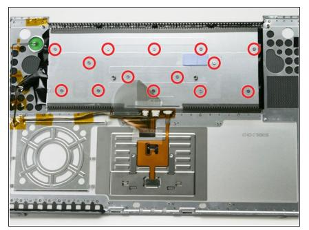
• Remove the 14 identical Phillips screws that attach the keyboard to the metal casing.
