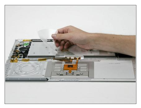
• Peel off the adhesive covering the back of the keyboard.
