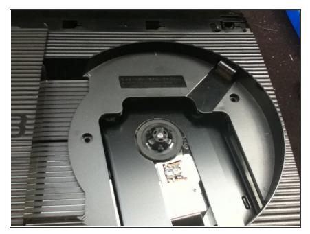
Remove two screws from the disk tray to remove the top.
