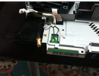
Remove the wireless aerial from the motherboard so that you can replace with a toggle antenna.
