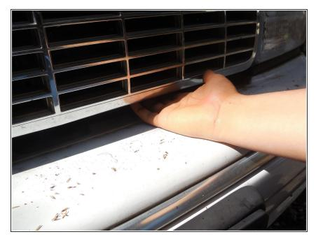
Go to the front of the car and push the lever up to unlatch the hood, you may need to feel around for a minute to find this.
