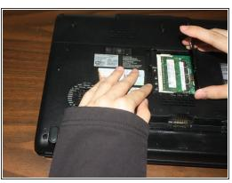
Unscrew the RAM cover and rotate the cover up to remove it. The screw should not be fully removed from the cover itself.
