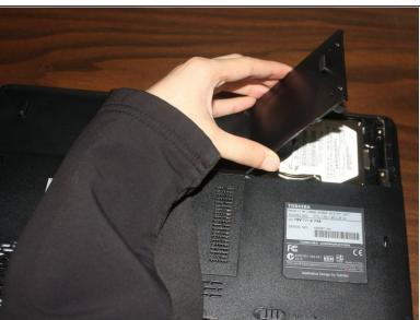
Unscrew the screws enough to remove the top cover.
