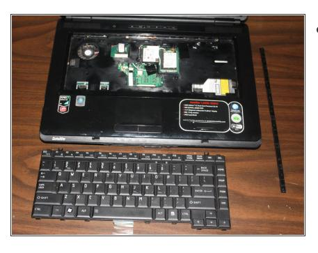
Remove the keyboard completely from the laptop.
