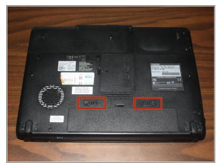
Locate the two sliding battery locks on the underside of the laptop.
