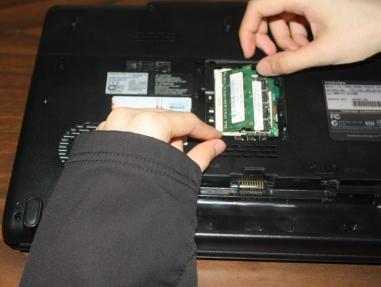
Push the small levers at the sides of the RAM module away from each other. The RAM module should automatically rotate upwards.
