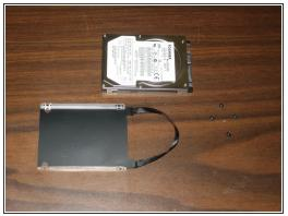
• To separate the hard drive from the caddy, unscrew the two screws.
