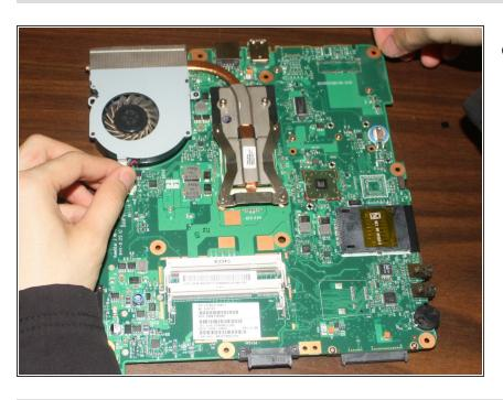
At this point the motherboard can be fully removed from the laptop.
