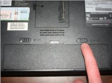
Locate the right battery lock and slide it to the right.
