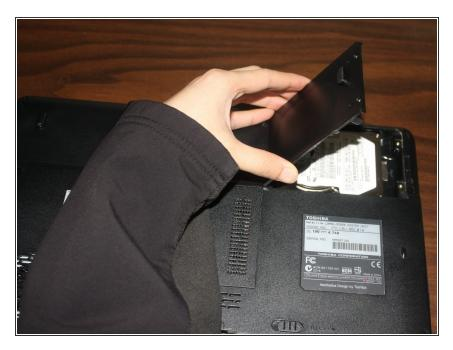
Remove the cover by lifting the right side up at an angle before removing the entire cover.
