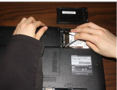
Remove the hard drive from the SATA slot by tugging lightly on the ribbon cable to the right.
