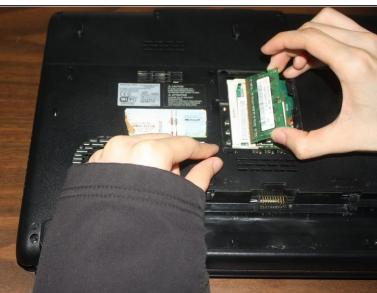
Remove the RAM module by pulling it out at the angle it was rotated to.
