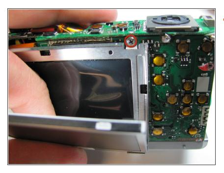
Remove the screw underneath LCD screen with the Phillips #00. The screw measures 4.1mm in length.
