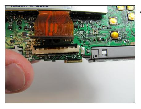
Remove the LCD ribbon cable from inside the black tab.
