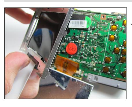
After desoldering the LCD casing, just use your fingers to carefully remove it.
