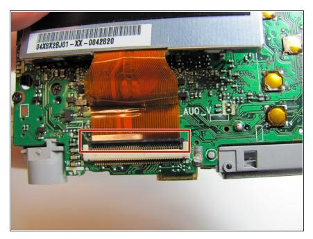
Flip up the black tab on the bottom of the LCD screen with a fingertip.
