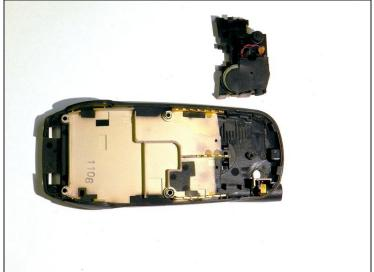
With the flat head screwdriver, remove the external speaker unit.
