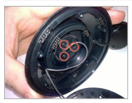
Remove the three 6 mm screws on the inside of the ear cup.
