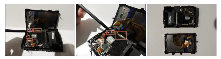
Using the spudger and tweezers if needed, remove the ribbons from the computer chips.
