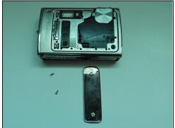
• Using the Phillips #00 screwdriver, unscrew the two screws on the side of the camera.
