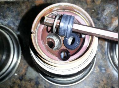
Remove seat assembly using an allen wrench or phillip head screwdriver
