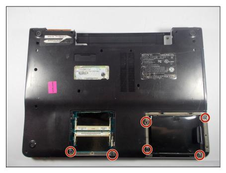
Remove the highlighted screws underneath the removed panels using the Phillips #0 Screwdriver.
