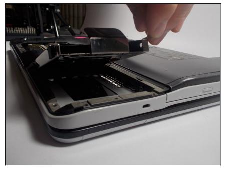
• Carefully remove the hard drive from the panel in the bottom right-hand corner of the laptop.
