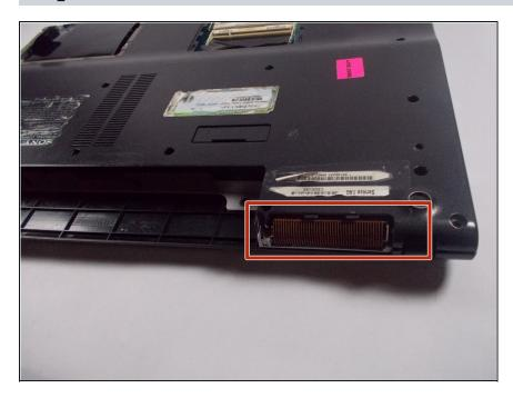
Remove cover in the top left side of the laptop next to the battery by pulling it outwards.
