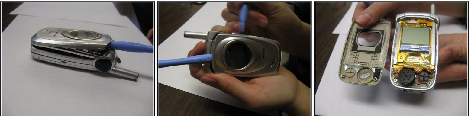
**⚠** The small electronic components inside the phone are fragile; take care not to damage them when completing this step.
