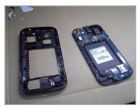
Here you can see the bottom casing separated from the top, now exposes the motherboard.
