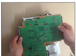
Remove the two heat sink clamps and bottom shield, then gently separate the motherboard off the top shield.
