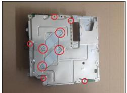
Disconnect the fan cable and remove the nine screws from the bottom side.
