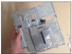
• Remove the four Phillips screws and lift the top shield.
