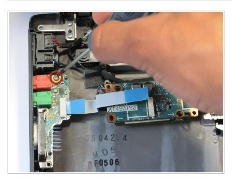
Remove the screws for the second ethernet circuit board.
