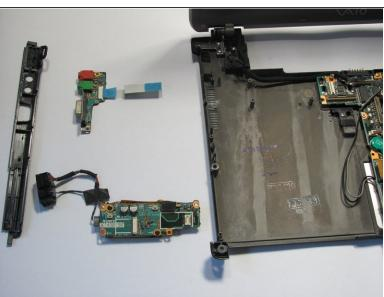
Remove the ethernet ports.
