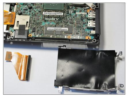
Remove the casing and the orange ribbon.
