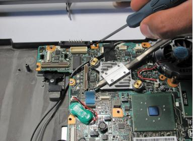
Remove screws on the motherboard.
