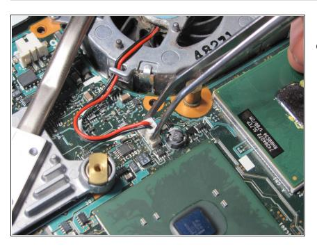
Disconnect the fan wire from the logic board
