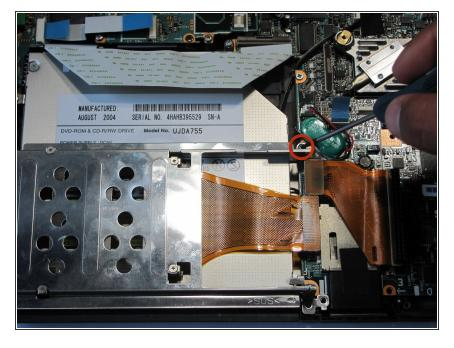
Remove the screw holding the optical drive casing to the logic board.
