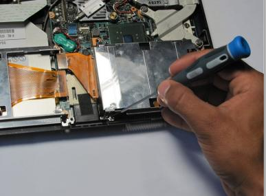
Remove the screws holding the hard drive casing in place.
