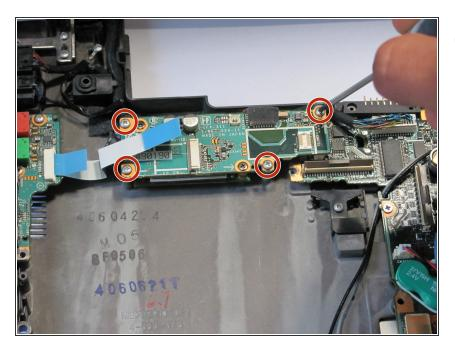
Remove the screws near the Ethernet Port circuit board.
