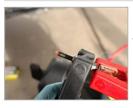
Shown here is a used glow plug that is not working quite right, despite glowing at the tip. The tip was slow to light compared to the new plug. You can also see that it is covered in carbon; it's a reminder that you'll want to ream the glow plug hole in the pre-chamber before installing a new one.
