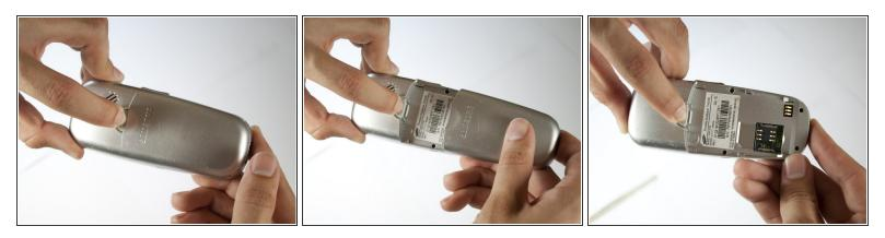
• Remove the battery by pressing down on the battery release button while sliding the battery downwards.
