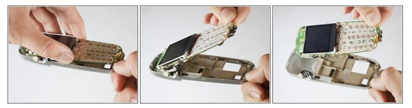
• Gently remove the logic board and LCD screen from the back cover of the phone.
