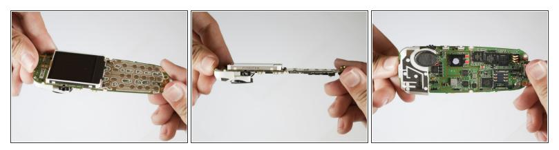
• Rotate the logic board so that the LCD screen is face down.
