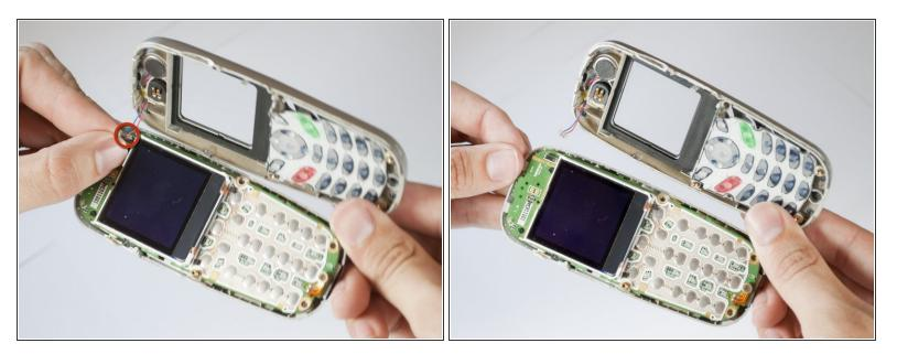
Using your nails, tweezers, or any precise grabbing tool, pinch the antenna wire connector (clear plastic plug) and pull gently. It should pop out rather easily.
