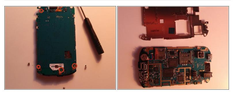
Remove the 5 screws to remove the shield
