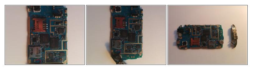
• Remove what seems to be the antenna from the logic board
