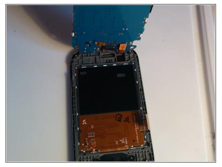
Remove logic board from screen by lifting the logic board up and removing the digitizer connector
