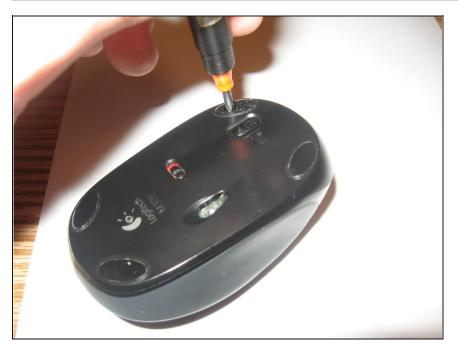
After removing all four sticky pads, unscrew the four screws.
