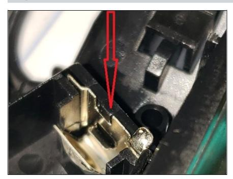
Battery contact on front of mouse (while the mouse cover is upside down). The red arrow is pointing to the black plastic tab holding the battery contact.
