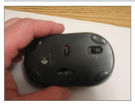
Turn mouse over to reveal the battery cover removal button.
