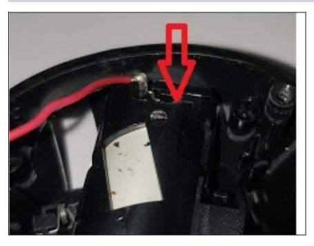
Battery Contact on the rear of mouse. There is a black plastic tab that holds the battery contact. The red arrow is pointing to it.
