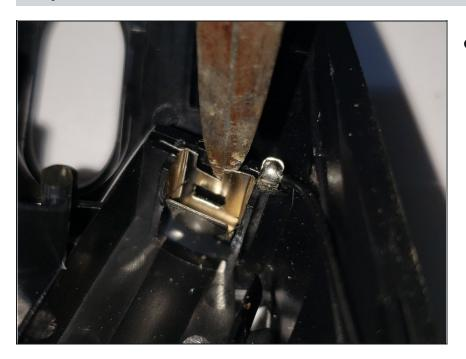
Tool is being used to pry the battery contact away from the black plastic tab. (please excuse the rough looking tool i used). Once the contact is pried away then take a pair of needle nose pliers and pull the battery contact straight up. You may have to wiggle the pliers some as you pull up.
