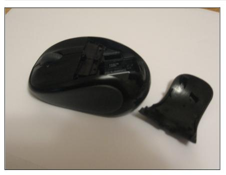
Slide the button back and then release in over to remove battery cover on the top of mouse.
