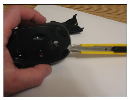
Remove (gently) sticky pads with the spudger or a sharp knife/cutter.
