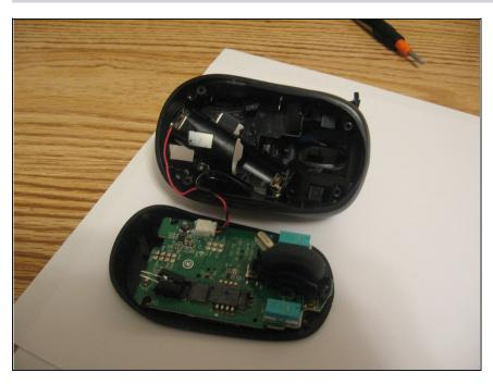
Once screws are removed, the top comes off, but be careful not to pull too hard because of the attached wires.
