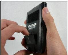
• Turn the device over so it is face down and remove the stylus, and battery cover.
