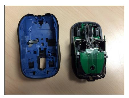
Lift the rear of the top case of the mouse and slide forward. It should be fairly easy to release.
