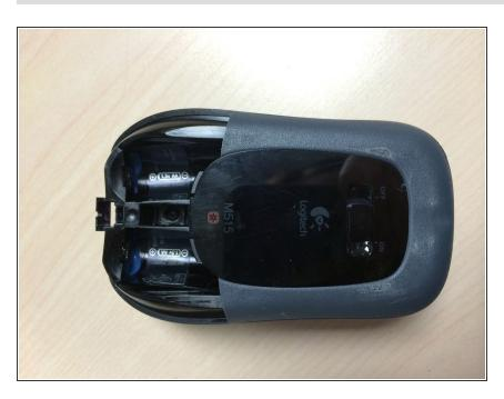
Remove the battery hatch and batteries.
