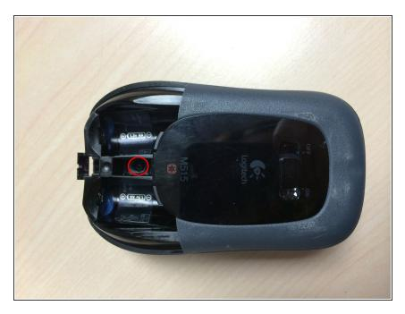
Remove the single Phillips screw located between the battery sockets.
