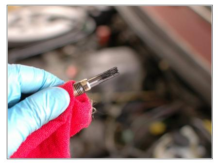
• Here is what the reamer pulled out of the #1 pre-chamber at the front of the engine.
