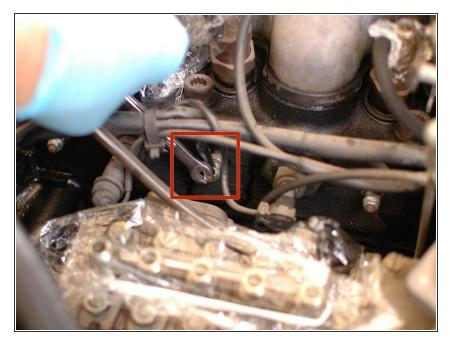
Begin by removing the small nut that holds the wire to the top of each glow plug. Use an 8mm wrench.
