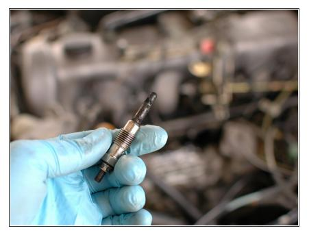
• Once removed you can inspect and test the glow plug to see if it was the one that was faulty.
