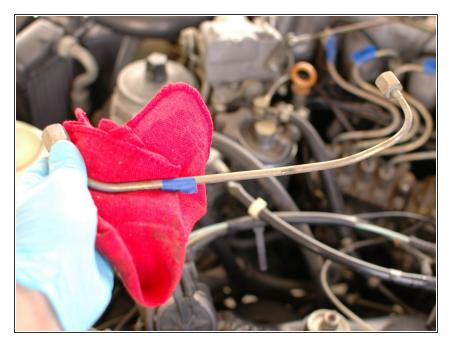
To make this job much easier, consider removing your injector hard lines. It makes it easier to get the correct tools on the glow plugs for removal. For guidance on this, <u>see</u> <u>the injector hard line removal guide.</u>
