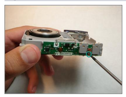
Remove screw from top of the flash mechanism
