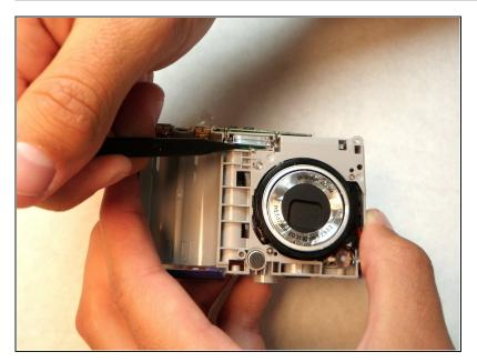
Remove the flash bulb from the camera housing by gently pulling on the wires with a pair of tweezers.
