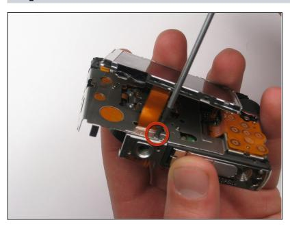
Remove the last screw holding the tripod mount to the case.
