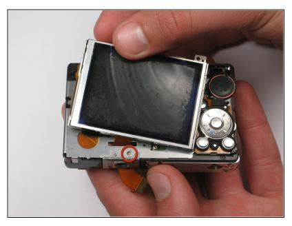
• Lift up the screen to reveal the tripod mount screw.
